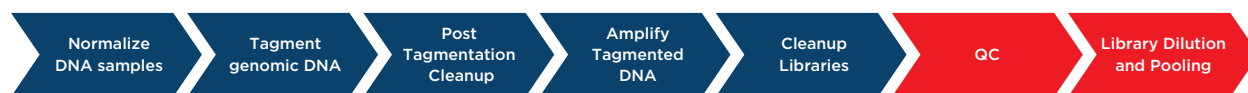
Figure 1. Workflow for Illumina DNA Prep protocol on the Biomek NGeniusS system. The blue arrows indicate the steps that are done on the instrument; the red arrows indicate the steps that are not.
